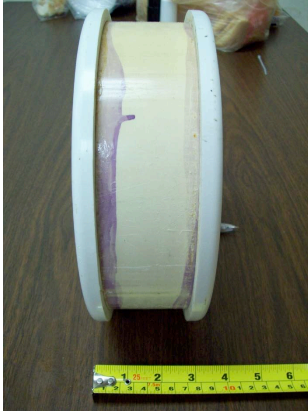
8" (Diameter) PVC pipe with 2 - 8" (Diameter) PVC coupler. Fully assembled Porthole.
